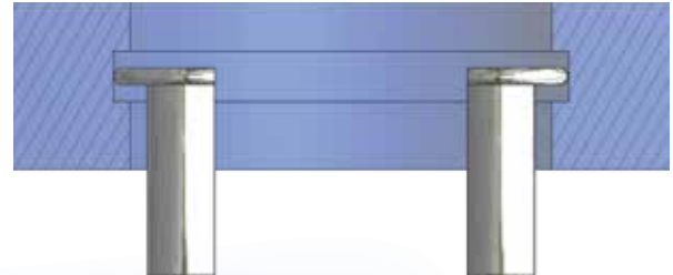
Messen einer Innennut Measuring of internal recesses
