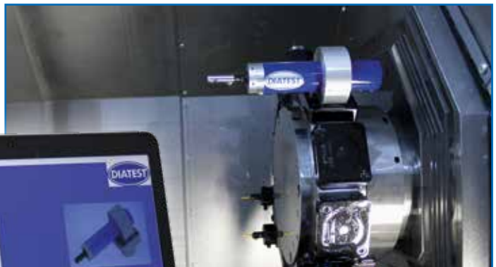
BMD in CNC-Drehmaschine Plug gauge BMD in CNC turning machine
