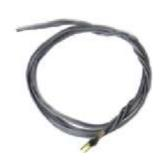
PTC Thermistors are semi conductor sensors. These have typical characteristics that change their resistance instantly at a specified pre-defined response temperature (NRT). As soon as the surrounding temperature of PTC reaches it's NRT value the body resistance of PTC Thermistor rises sharply from 200 / 250 Ohms to more than 5000 Ohms.
