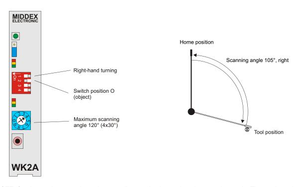
NOTE: Set the maximum angle on the controller equal or larger than the scanning angle. The teach-angle area equals the selected angle plus approximately 5°.
